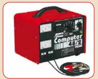
COMPUTER 48/2 PROF 230V 6--48V Single-phase, portable, professional battery charger for charging all types of batteries with 6/12/24/36/48 v voltage. With automatic protection against overloads and polarity reversal. Allows simultaneous charging of several batteries in series. Equipped with ammeter and voltmeter.
