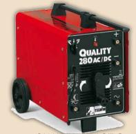
QUALITY 280 AC/DC MMA stick electrode welding machine in direct (DC) and alternating current (AC). Stepless regulationof welding current. With thermostatic protection. Use with a wide range of electrodes: rutile, basic, stainless steel and cast iron
