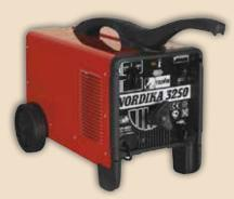
Nordika 3250 230-400v Single-phase, on wheels, fan-cooled stick electrode welding machine for mma welding in alternating current (ac). Stepless regulation of welding current. With thermal protection. Usable electrodes: rutile.
