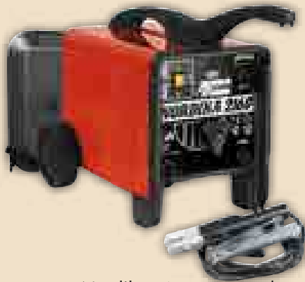
Nordika 2160 230v ac Single-phase, on wheels, fan-cooled stick electrode welding machine for mma welding in alternating current (ac). Stepless regulation of welding current. With thermal protection. Usable electrodes: rutile. Complete with welding accessories.
